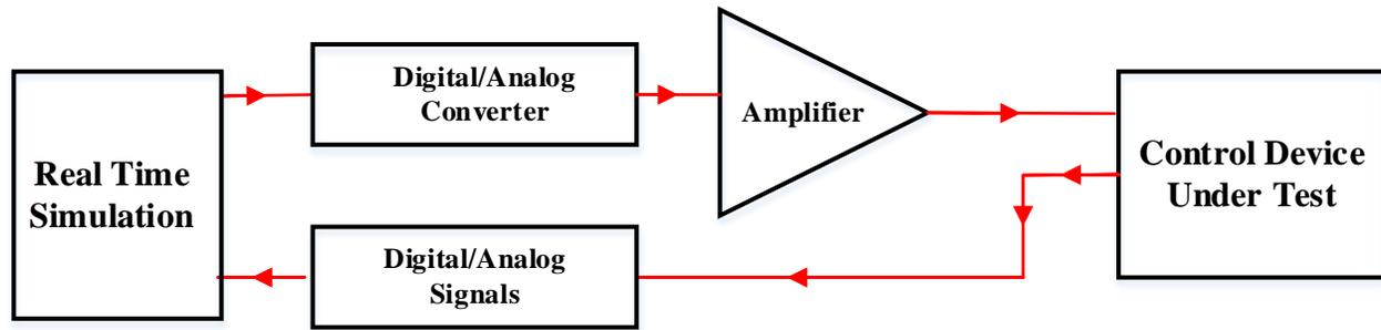
Figure 1-1 Control Hardware In the Loop (CHIL) simulations
