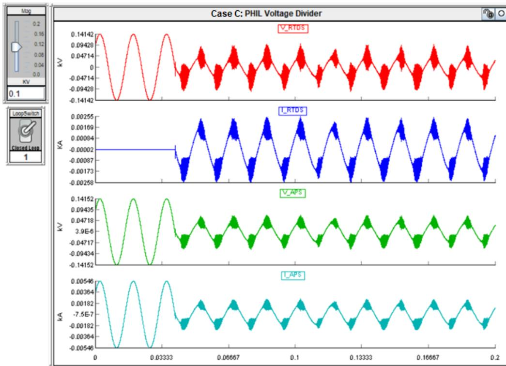
Figure 3-20 Case C: Transition from open to closed loop simulation results (unstable)
