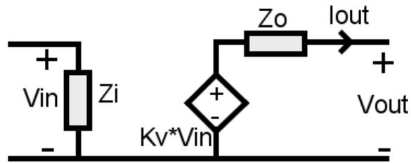
Figure 2-11 Controlled Voltage Amplifier
