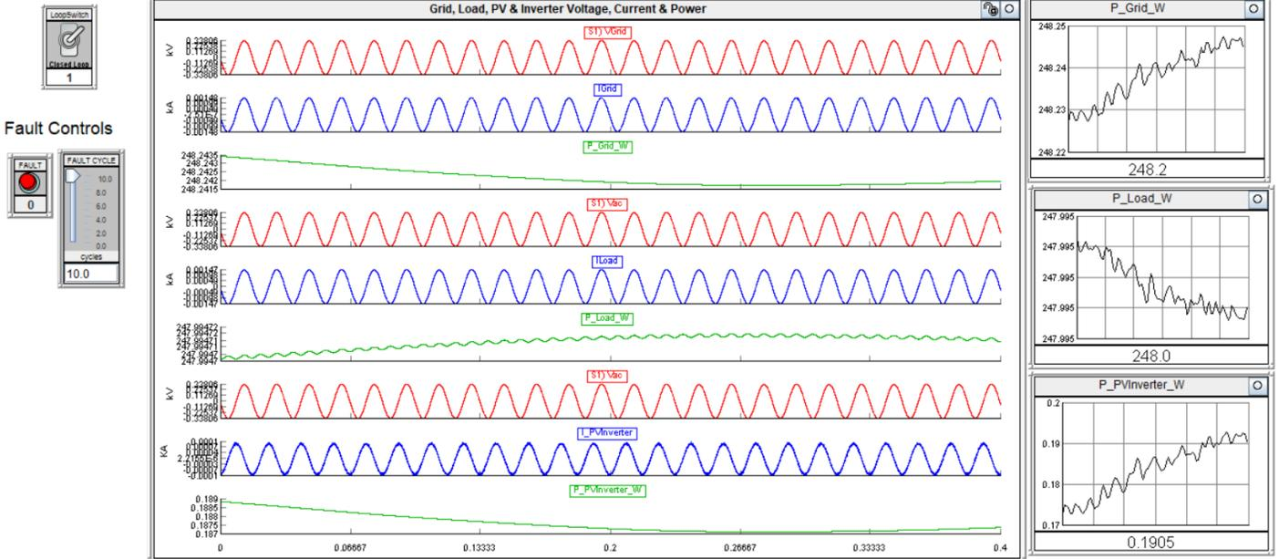
Figure 4-4 Grid, Load, PV and Inverter Voltage, Current & Power (Prior to Inverter Start-up)
