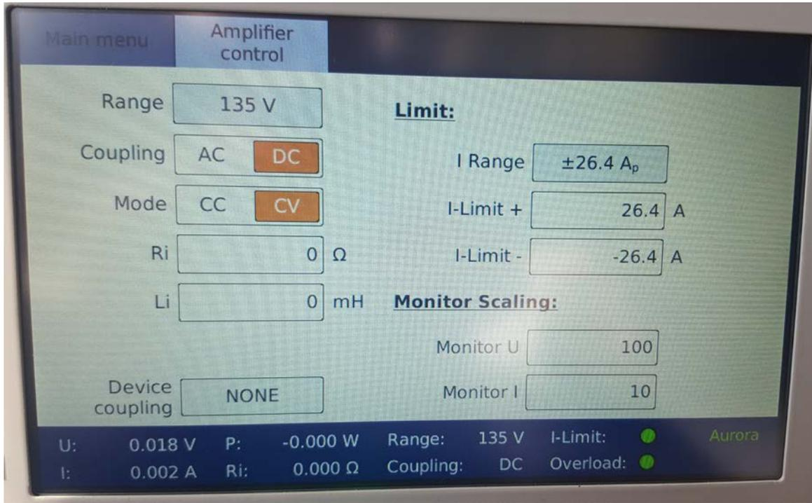
Figure 3-8 APS 1000 Amplifier Control settings
