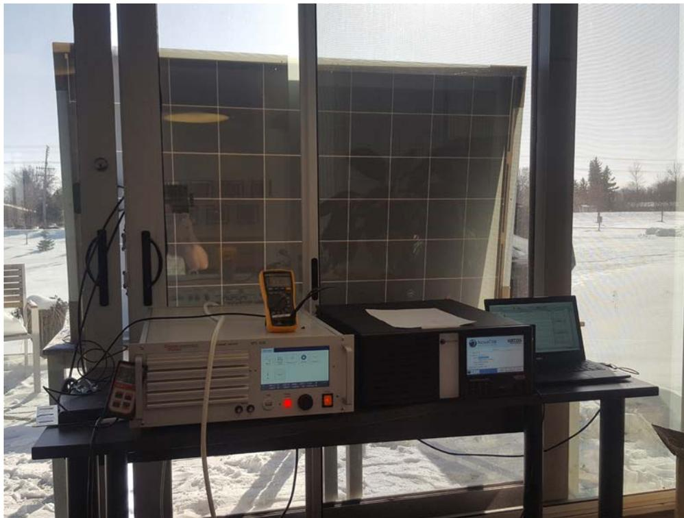
Figure 4-1 PHIL interface with PV inverter
