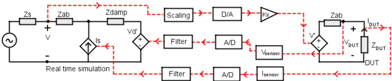
Figure 2-9 Damping Impedance Method (DIM)
