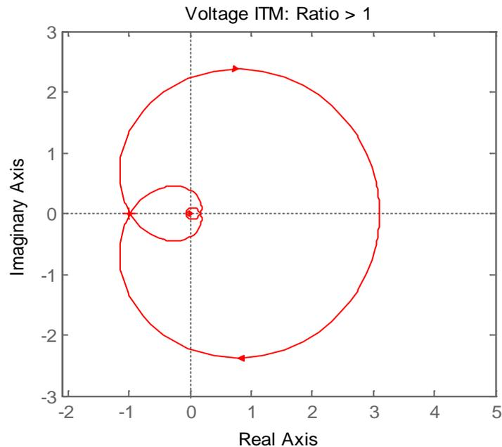
Figure 2-4 Nyquist Contour for Voltage Type ITM
