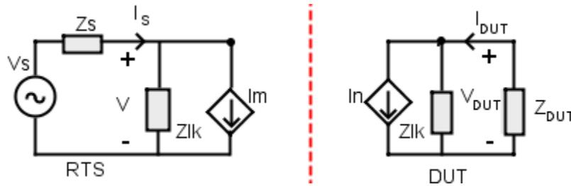
Figure 2-7 Transmission Line Method (TLM) - Norton Equivalent
