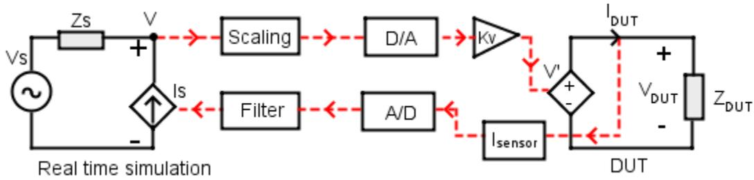
Figure 2-2 Voltage Type: Ideal Transformer Method
