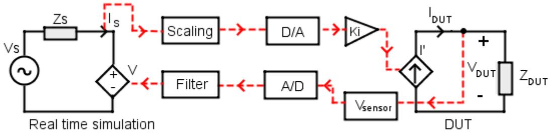
Figure 2-3 Current Type: Ideal Transformer Method
