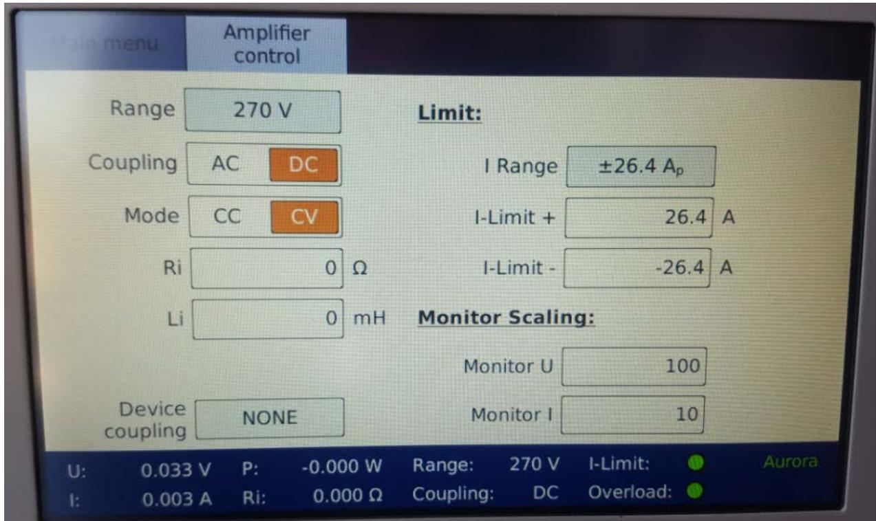
Figure 4-2 APS 1000 Amplifier Control settings
