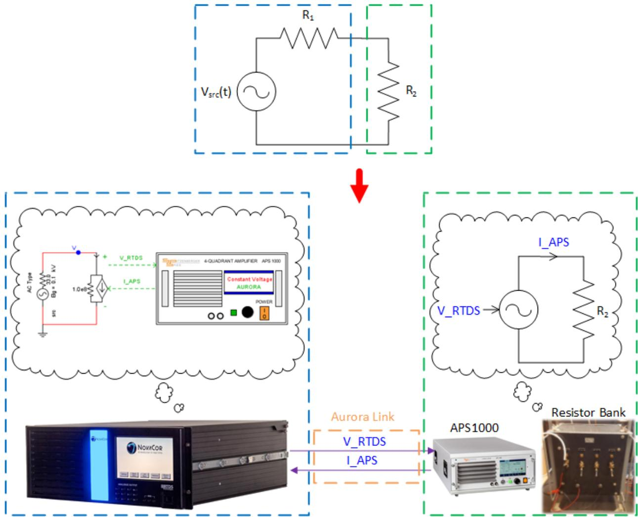
Figure 3-7 PHIL ITM interface for voltage divider circuit
