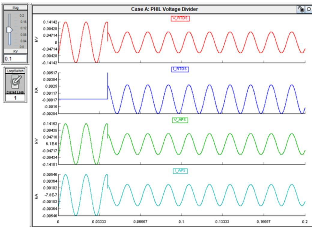
Figure 3-12 Case A: Transition from open to closed loop simulation results
