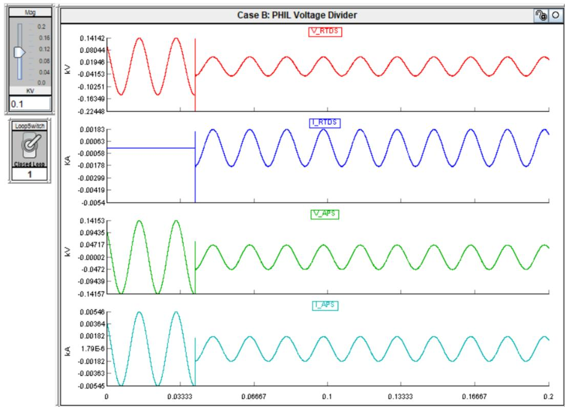
Figure 3-16 Case B: Transition from open to closed loop simulation results
