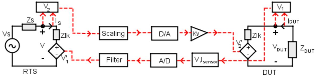
Figure 2-6 Transmission Line Method (TLM) - Thevenin Equivalent
