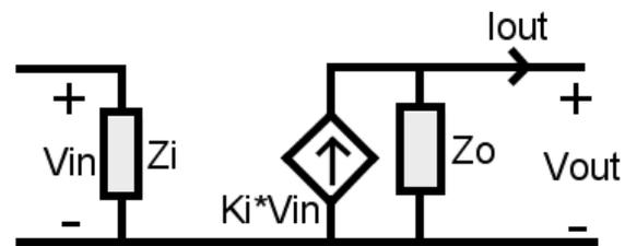
Figure 2-12 Controlled Current Amplifier
