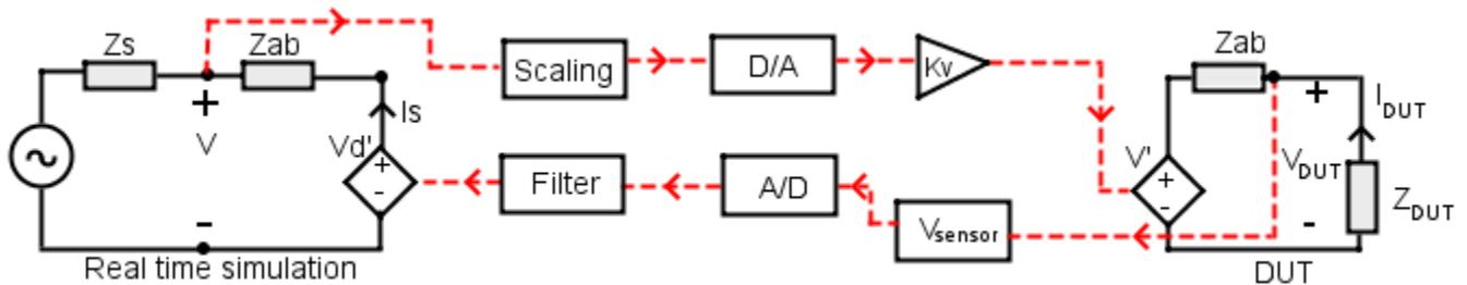
Figure 2-8 Partial Circuit Duplication (PCD)
