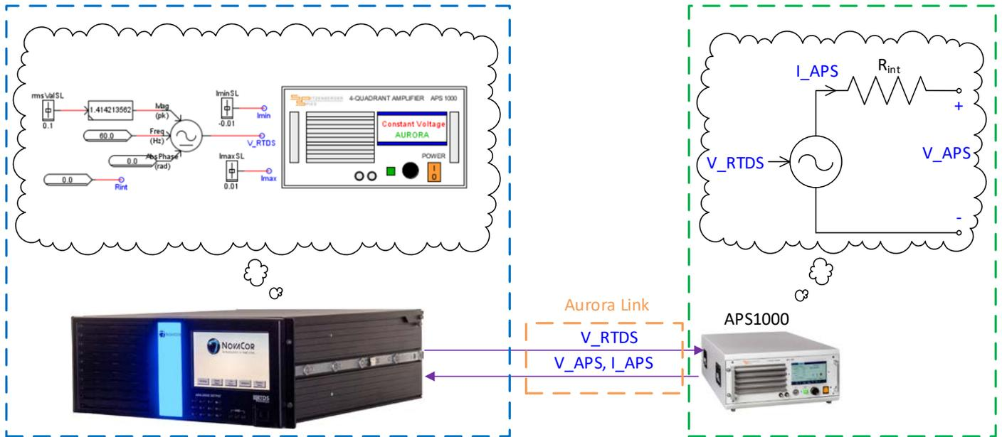
Figure 3-1 Interface noise test setup
