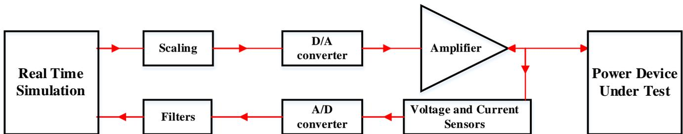
Figure 2-1 Power Hardware In the Loop (PHIL) simulations
