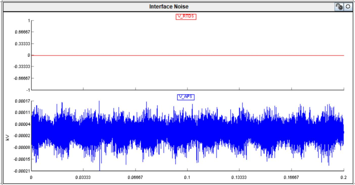
Figure 3-5 Interface noise for voltage measurement (Zoomed out)
