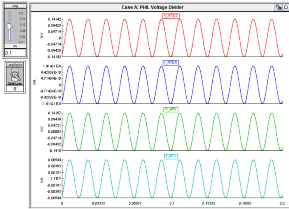
Figure 3-11 Case A: Open loop simulation results
