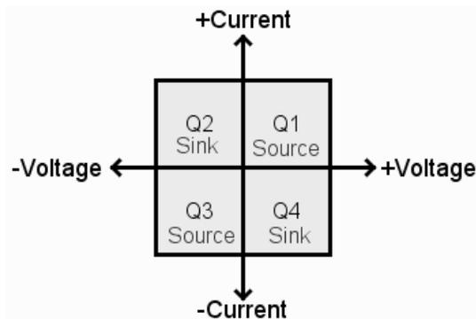
Figure 2-10 Four quadrant amplifier operation for PHIL simulations
