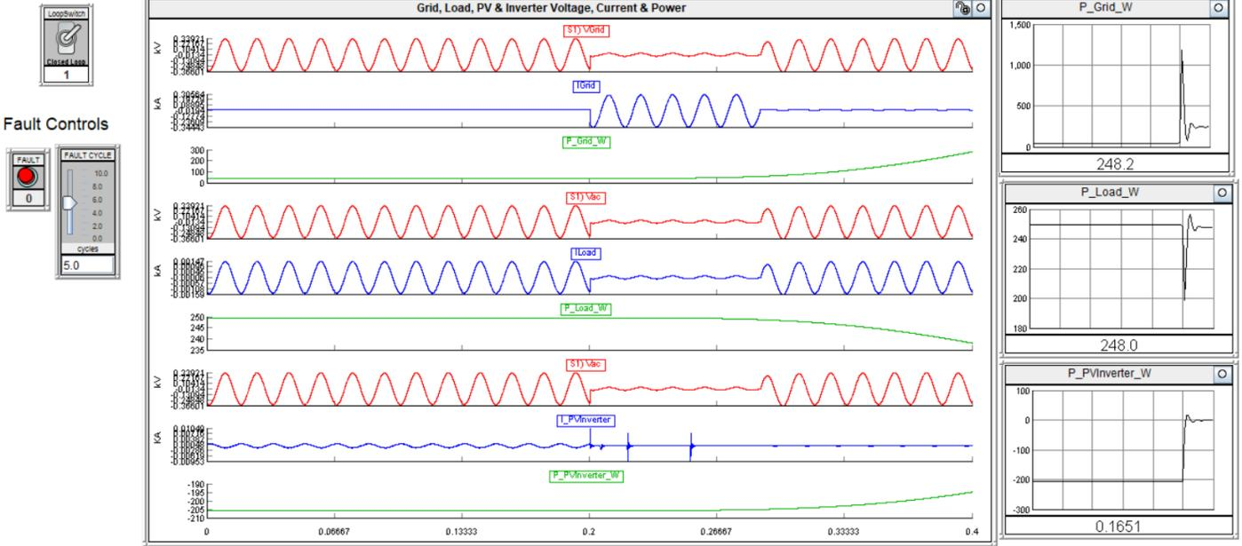
Figure 4-8 Grid, Load, PV and Inverter Voltage, Current & Power (5 Cycle LG Fault)
