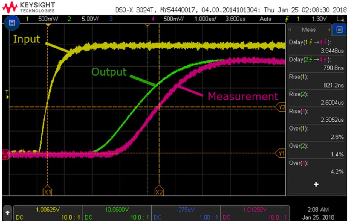
Figure 2-15 Amplifier step response
